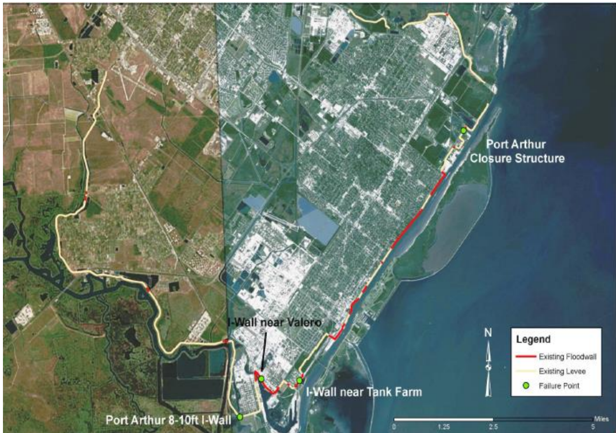
Figure 3-4: Port Arthur and Vicinity CSRM Failure Locations
