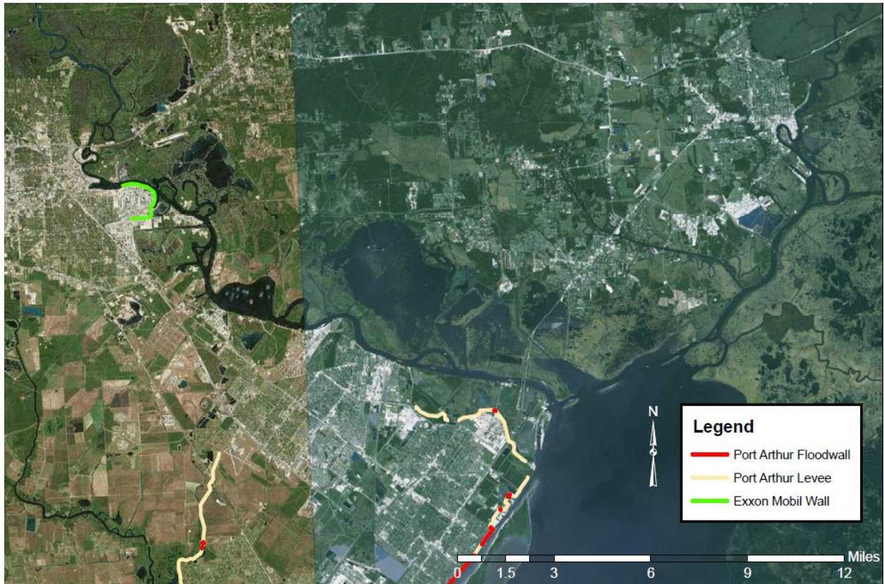
Figure 3-3: Existing Floodwall in the Orange-Jefferson CSRМ Project Areas
