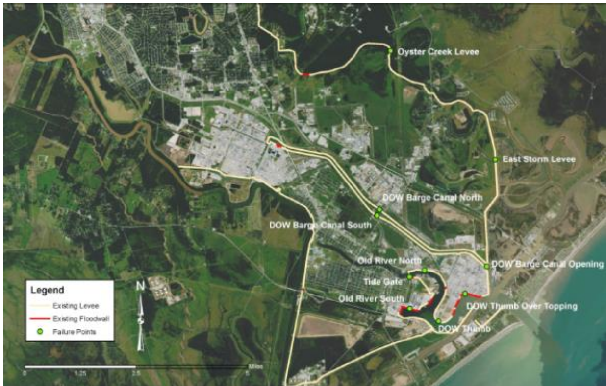
Figure 3-8: Freeport and Vicinity CSRM Failure Locations
